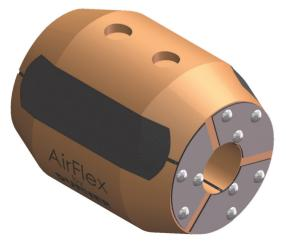
To protect the rubber of the AirFlex guide bush against the high pressure coolant mixed with chips, it's possible to add HP protective shields. These shields are made on steel and help to increase lifetime of your guide bush.
